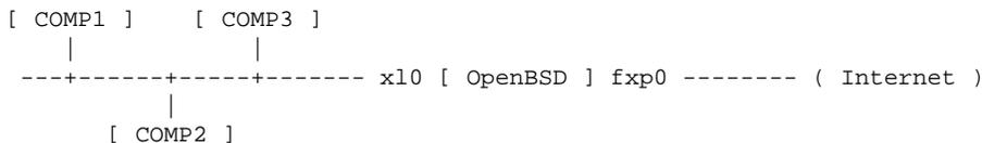
There are a number of computers on the internal network; the diagram shows three but the actual number is irrelevant. These computers are regular workstations used for web surfing, email, chatting, etc., except for COMP3 which is also running a small web server. The internal network is using the 192.168.0.0 / 255.255.255.0 network block.
