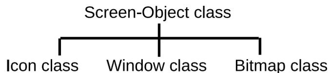
Figure 3.9. The Screen-Object Superclass
