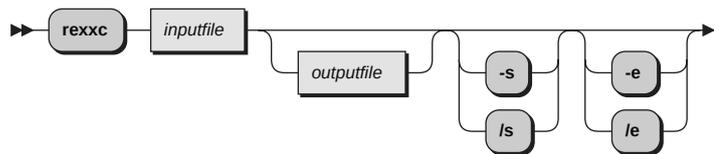
If you specify the `outputfile`, the language processor processes the `inputfile` and writes the executable version of the program to the `outputfile` (a binary file). If the `outputfile` already exists, it is replaced.
